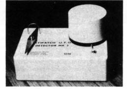
A magnetic needle type detector incorporating a solid state latching circuit and audio alarm. Battery operated.
