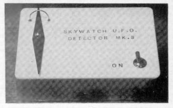
A magnetic needle type detector incorporating a solid state latching circuit for the audio alarm. Battery operated.
