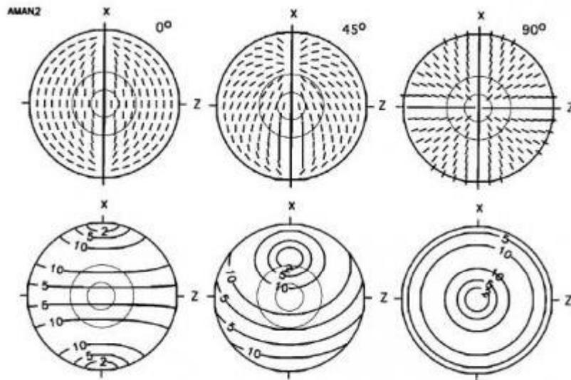
Fig. 4. Examples of shear stress patterns for horizontal and vertical plate movement.
