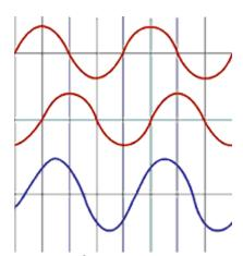
Two waves added out of phase give an intermediate wave.
